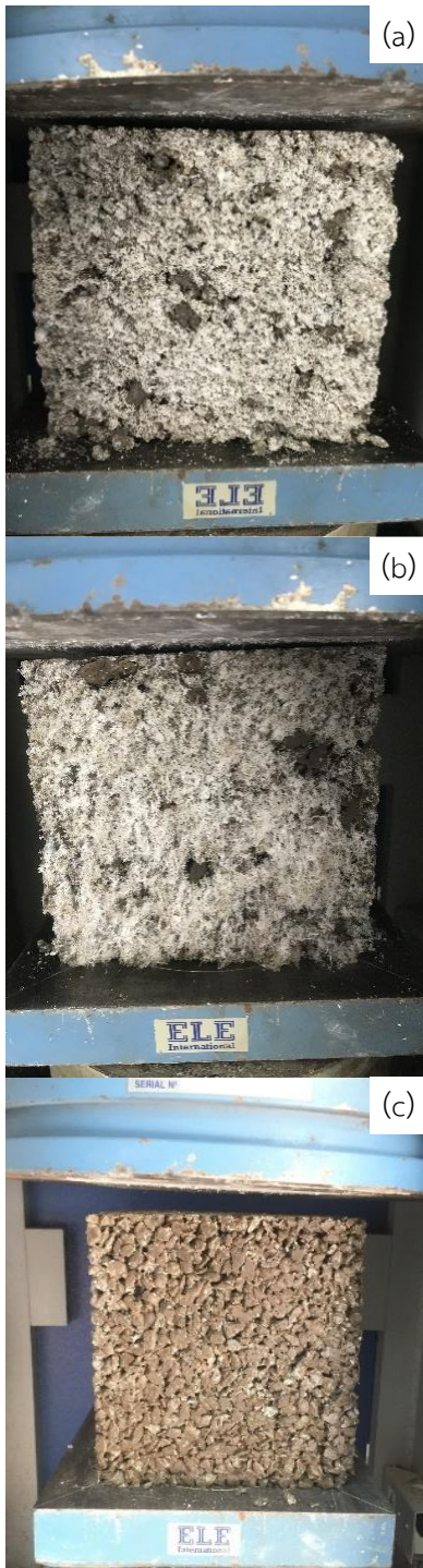
Figure 4 Physical properties of pervious geopolymer concrete at 28 days (a) 1:25 (b) 1 and (c) 0.75
